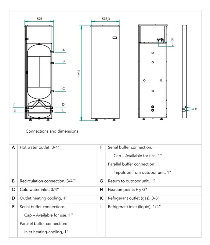
\* It's possible to leading the F and G connections through the gaps obtained by releasing the fixation points.
