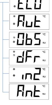
ECO Mode: Heating only by heat pump technology
