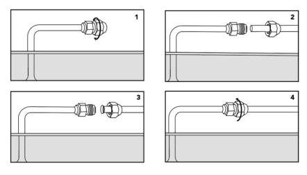
Then, join the suction line that comes from the panel to the coolant inlet of ECOHEAT, and the liquid line to the coolant outlet. The connections are threaded, if welding is needed, weld by oxyacetylene welding.
