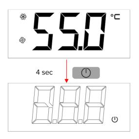
To switch off the system, hold the key for 4 seconds.
